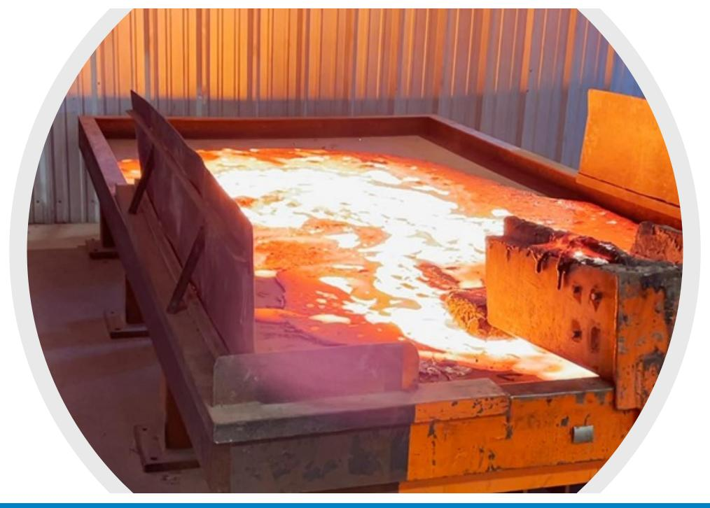
Slag from a tap is richer in PGM's than overflow slag so it is processed, milled and returned to the furnace for additional smelting
