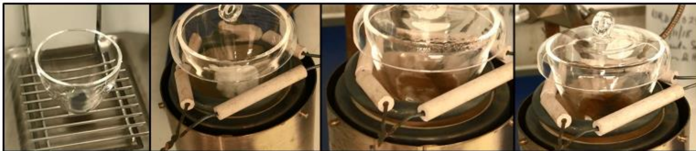
Sample Os 0 weighed into quartz crucible
