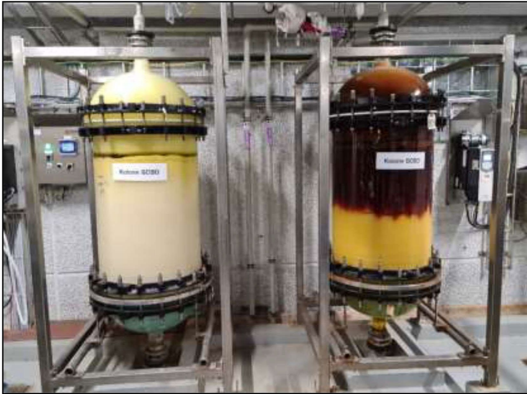
Figure 12. MRT™ Industrial Facility for Palladium Separation and Recovery at the Boliden Rönnskär Precious Metals Refinery in Sweden. The column on the left is packed with SuperLig® 2 resin beads. The column on the right is loaded with Pd (dark coloration.) Reproduced with permission from [46b].
